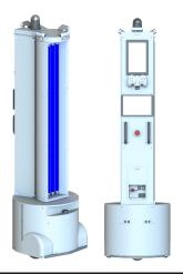
The Akara UV robot decontaminates hospital rooms using scientifically proven germ-killing UV light. Unlike other UV disinfection products, the device doesn't require rooms to be evacuated during use. This streamlines workflow and facilitates full room decontamination in more clinical settings.
