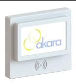
The Akara Hub is a wall-mounted computing device that tracks equipment in the room, issues digital notifications to staff, enables authenticated digital sign-off task checklists, and facilitates integration of Akara-approved smart devices with the hospital's building management system (BMS).
