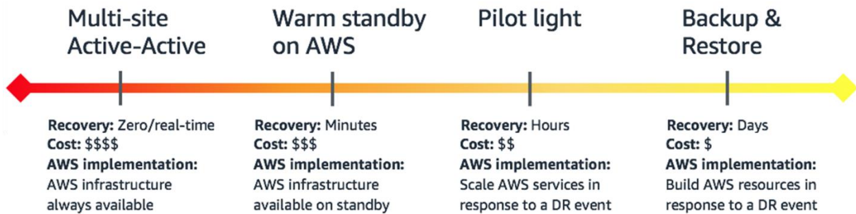
Figure 5. Spectrum of DR Options. Customers can choose a preferred DR option based on preferences for cost and the time it takes to recover systems.
