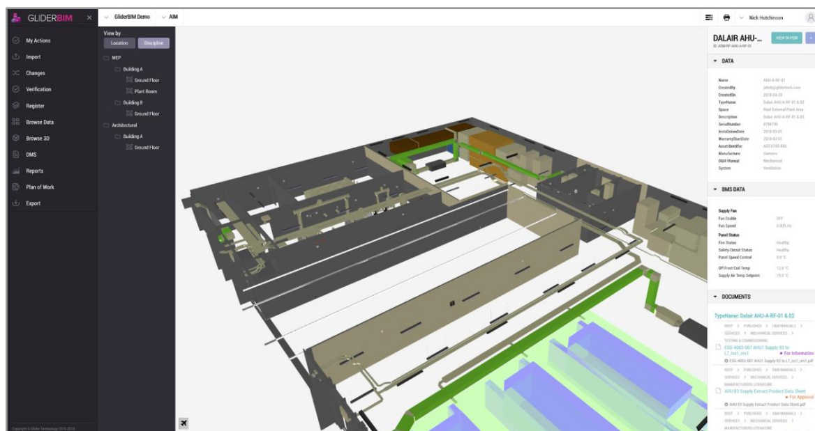
Figure 2 - Connecting geometric models with structured data and documents
